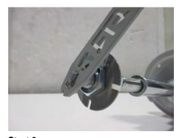
Strut 3: Using 0 as a reference point, each mark on the dial is a ¼ turn, every time you pass 0 is on full turn. The strut will rotate 2 1/4 turn from full soft to full stiff. It is suggested you start in the middle and adjust to firmer or softer depending on your vehicle's needs.
