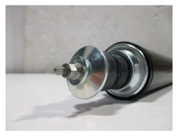
Shock 1: Begin with removing the shock nut. Then slide on the shock dial, loosely fastening the nut back on the shock.
