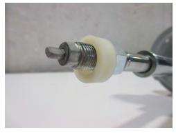
Strut 1: Begin with placing the supplied nylon bushing over top of the strut mount bolt followed by the strut dal then loosely thread on the supplied nut.
