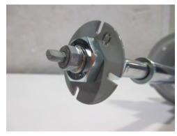
Strut 2: Using the supplied adjuster tool, use the F notch turn the strut clockwise until it stops. This is the softest setting. Rotate the dial to the 0 position at full soft and tighten the nut.
